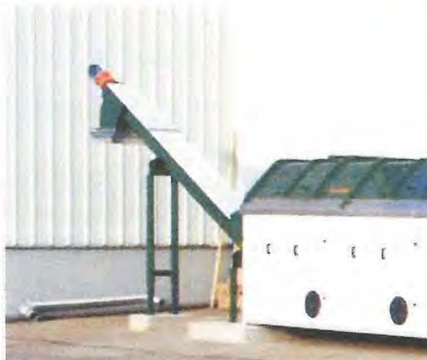
Incline discharge auger installed on smaller HotRot 1811 composting unit
